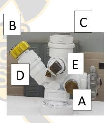
**POL** (Prest-O-Lite) port Adapter connected. Valve in closed position
