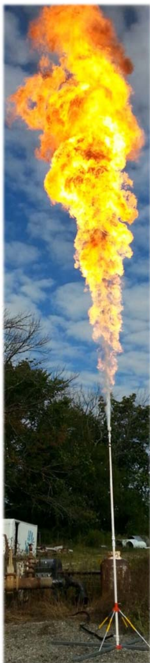
Figure 2 - 1" flare burning liquid
