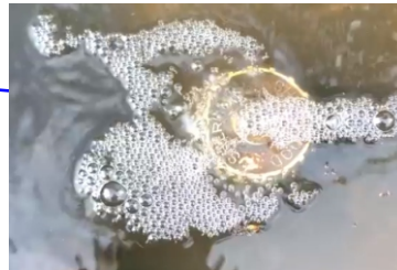
Upper O-Ring leak on underground tank
