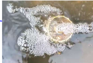
Upper O-Ring leak on underground tank
