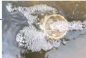
Upper O-Ring leak on underground tank
