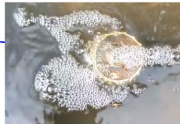
Upper O-Ring leak on underground tank
