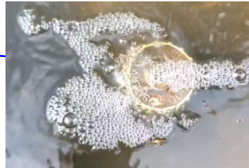
Upper O-Ring leak on underground tank
