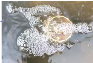
Upper O-Ring leak on underground tank
